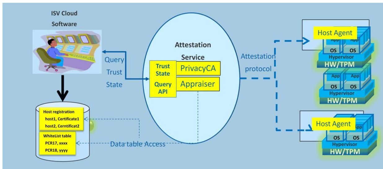
This above diagram highlights OpenAttestation architecture. OpenAttestation, as part of 3<sup>rd</sup> party ISV's software stack, enables ISV software remotely to retrieve and verify target
